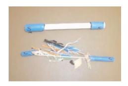
Image taken from an independent report commissioned to test the ARM@CORE cable performance. Top cable shows the ARM@CORE design. Outer Nylon sheath provides little resistance to rodent attack. However, the rodents cannot penetrate through the GRP armour and the inner core of the cable is left fully protected. Bottom cable is a conventional loose tube cable and is completely destroyed by the rodents.
