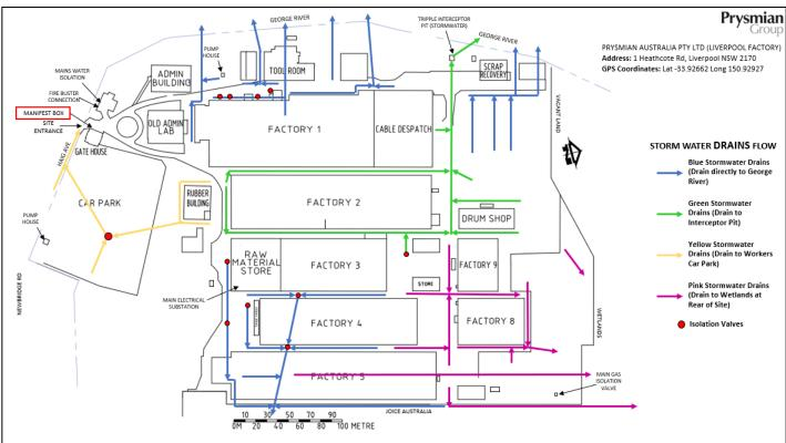
Figure 7-1: Stormwater Drains and Isolation Valves Layout
