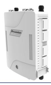
The Internal Flexibox is a wall box designed for internal use with 8 splice trays and up to 8 individual inputs for up to 24 cables. Each splice tray is able to accommodate 12 fibre splices and the box has a tube storage area. The Flexibox is available with a lock for security and also has a removable cover for extra access whilst splicing and routing fibres. The box has been designed to stack multiple Flexiboxes side-by-side, without compromising space.
